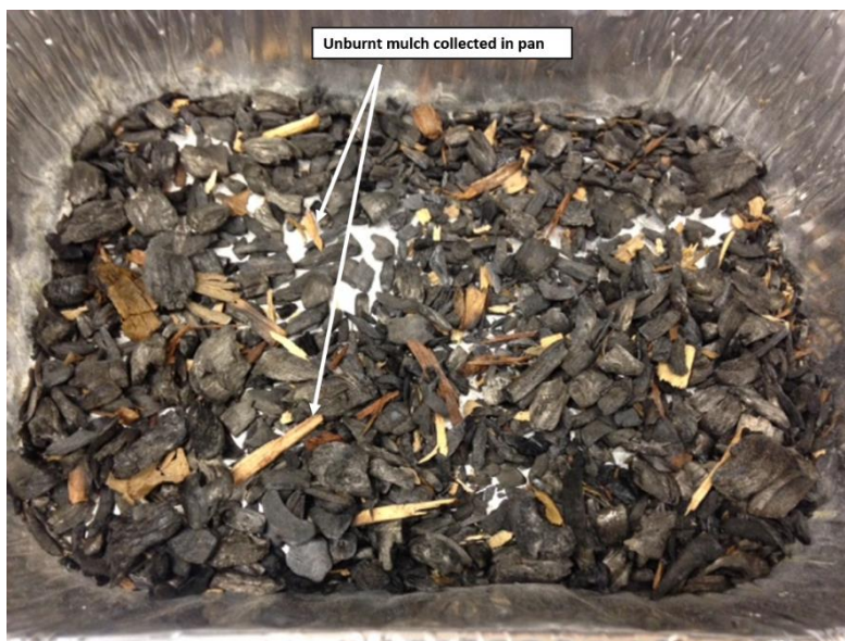
Figure 2 Collected firebrands in experiment with flap of 150 mm and high wind speed.
