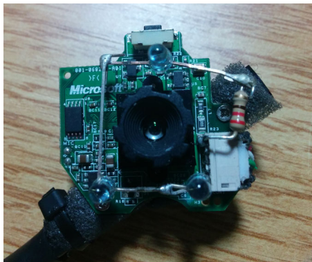
Figure 4.10: The webcam mounted to the aluminium wire.
