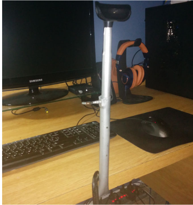
Figure 5.3: Height-adjustable chin rest to stabilise the head for eye tracking.
