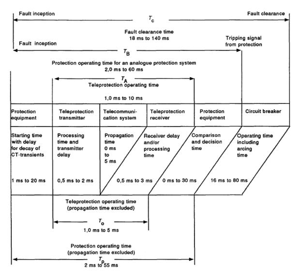
Figure 4.1 – Typical operating times for analogue comparison protection systems (IEC-60834-2, p.55)
