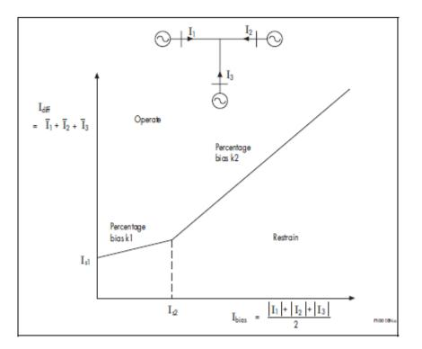
The characteristic is determined by four protection settings:
