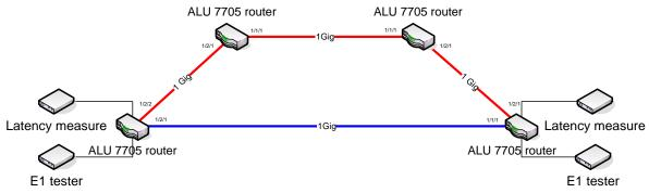
Figure 7.1 – Laboratory Testing Configuration
