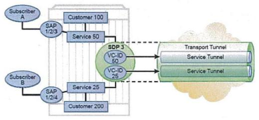
The transport tunnel for a service is represented by the SDP seen below in Figure 3.4.
