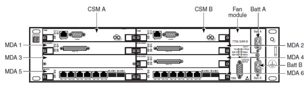
**Figure 6.1 – 7705 SAR-8 Front View** (ALU 7705 SAR-8 Chassis Installation Guide, 2013)
