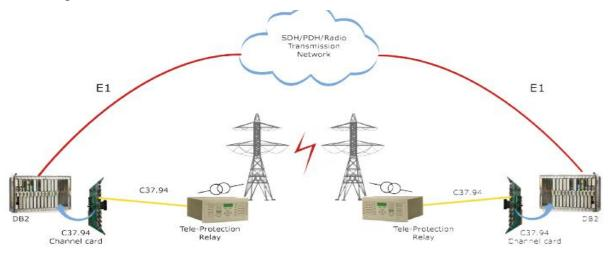
Figure 5.1 – Teleprotection-over-TDM network system (Avara C37.94 Optical Data Interface Unit, 2010)
