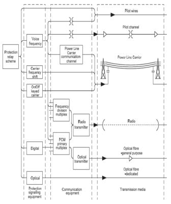
implementations of communications Figure 2.1 – Protection Signalling and Communications Systems (Alstom, 2011)
