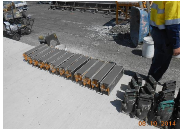
Step 4 – Full range of testing showing compression cylinders and flexural beams.
