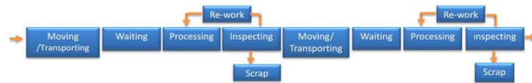
Figure 4 - Flow model applied to the transformation of materials repeated over two cycles. (Abeysekera 2009, p. 205)
