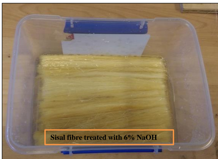
Fig.3. 3 Sisal fibre soaked in 6% NaOH solution
