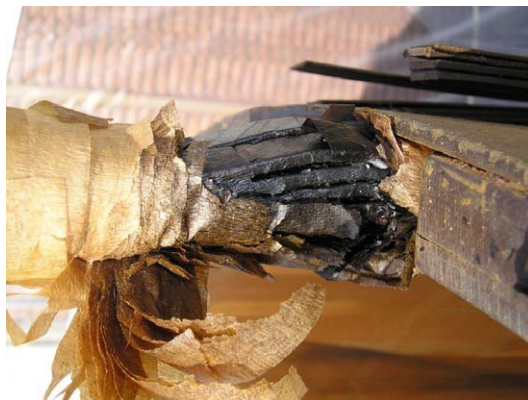
Figure 2.3: Extensive damage to paper insulation caused by pyrolysis (Cigré 2009, p. 16).
