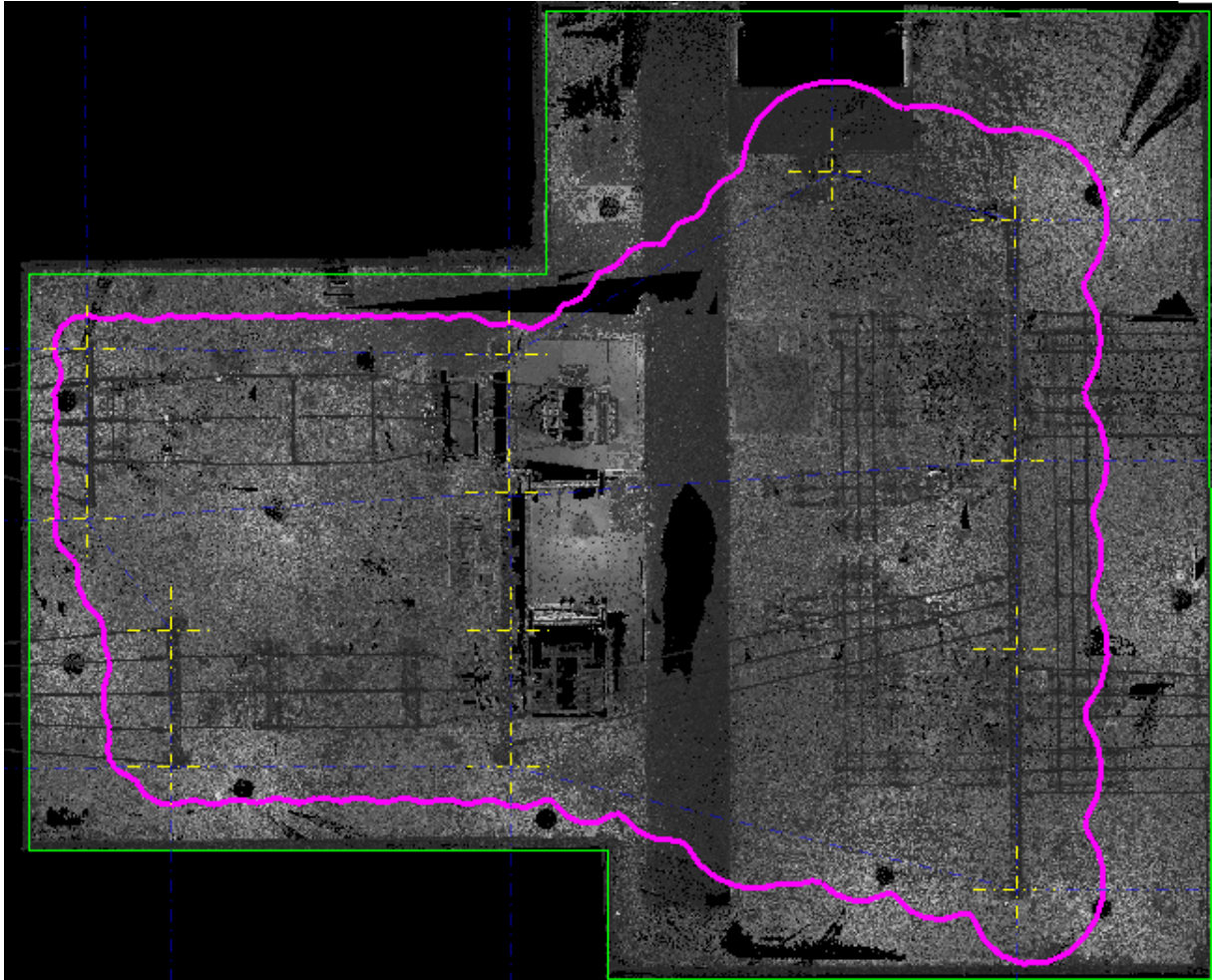
Figure 60: Plan view clearance area shown on point cloud file.
