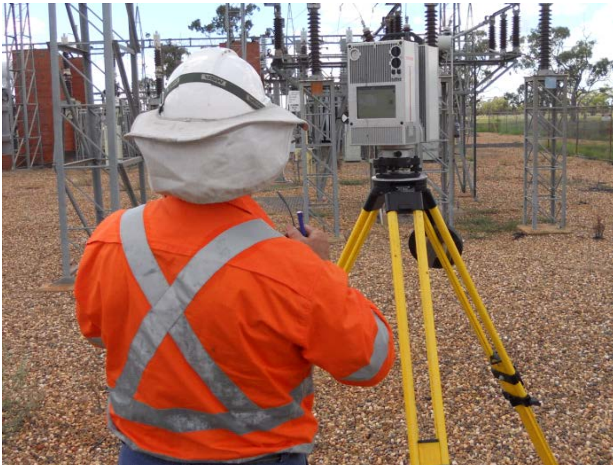
Figure 5: Operation of a TLS device.
