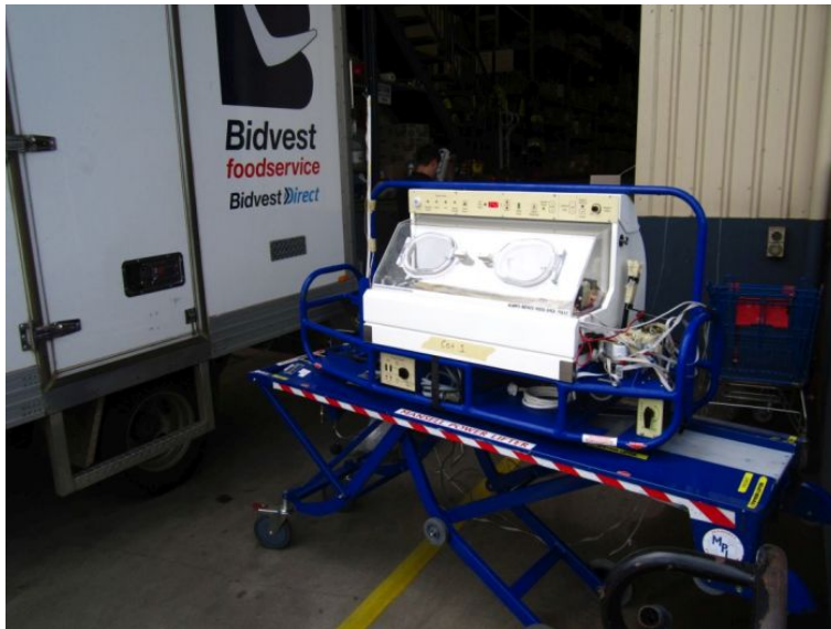
Figure 5.1: The Neocot just before the start of the cold test.
