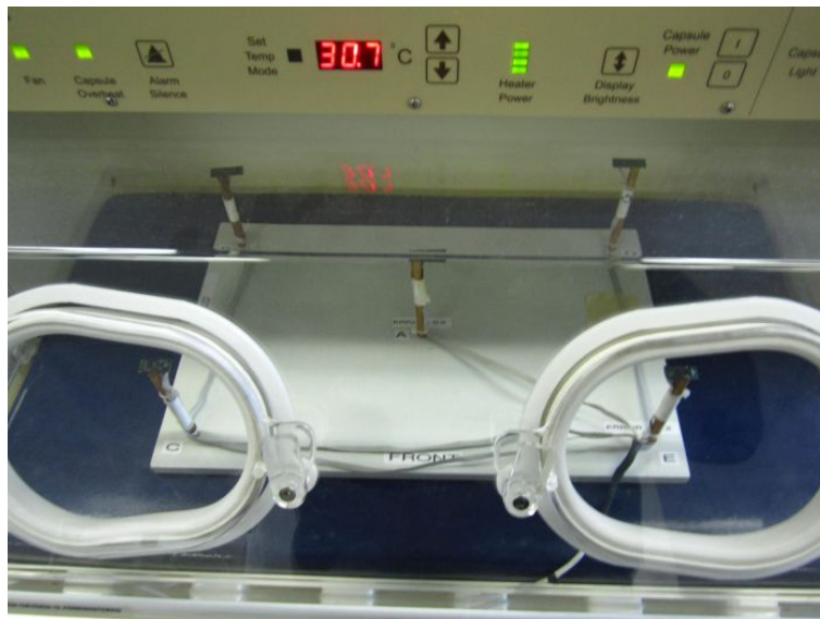
Figure 6.2: Five sensor array configuration within the Neocot.
