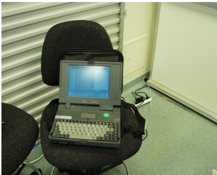
Figure 3.1: Laptop configuration for gathering of temperature data.
