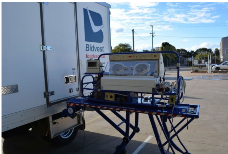
Figure 5.11: Neocot just prior to placing in cold truck with the LM35 external temperature probe placed inside.
