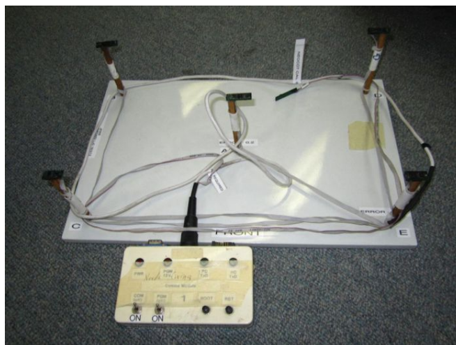
Figure 7.1: Five sensor array used for temperature logging of Neocot.
