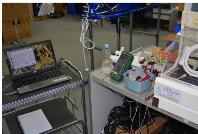
Figure 4.4: New calibration process, amplifier circuit and LabJack maintained in a temperature controlled environment.
