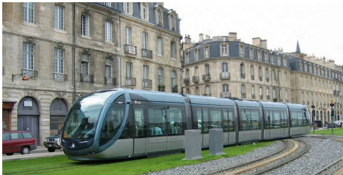
Figure 2.5 – Low floor tram on catenary-free section in Bordeaux
