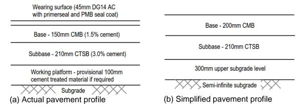
Figure 4-2 Typical pavement profile simplification adopted for back-analysis.
