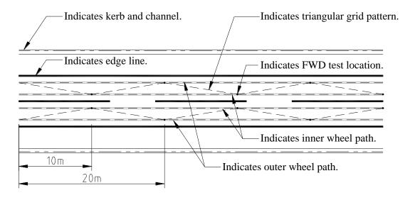
Figure 3-6 FWD proposed testing layout
