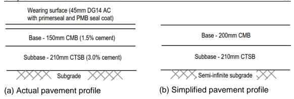
Figure 4-7 Typical pavement profile simplification for CIRCLY design analysis
