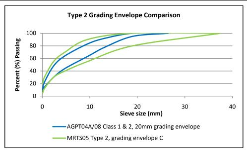
Figure 2-1 AGPT04A/08 and MRTS05 Type 2 grading envelope comparison.
