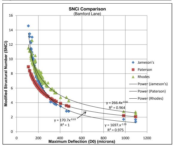
Figure 4-9 Modified Structural Number (SNC) method comparison
