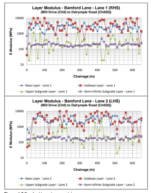
Figure 4-5 Bamford Lane layer modulus
