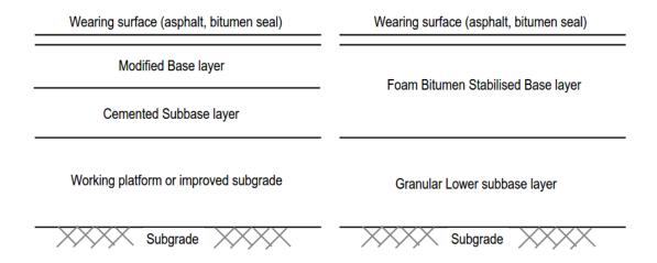
Figure 2-4 Example pavement structures
