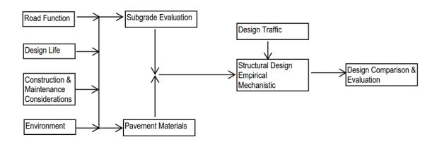
Figure 2-3 Pavement design process (Austroads, AGPT02/12)
