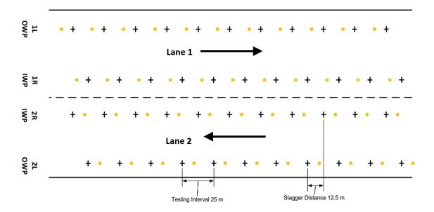
Figure 4-1 Typical FWD staggered testing layout.
