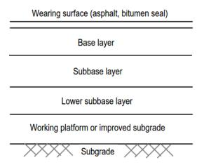
Figure 2-2 A typical pavement profile.
