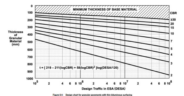
**Figure 2-5** Heavily trafficked (DESA 1x10<sup>5</sup> to 1x10<sup>8</sup>) empirical pavement thickness design chart (Austroads, AGPT02/12, Figure 8.4)
