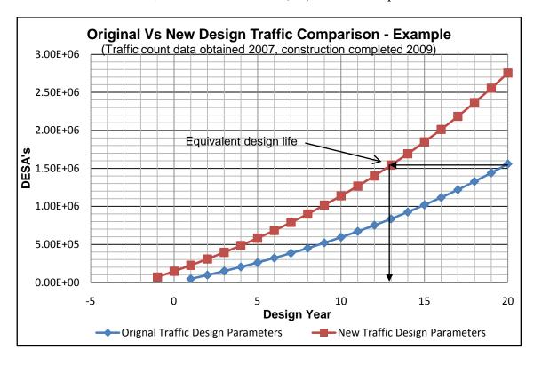
**Figure 4-8** Example of the effect of modified traffic design parameters
