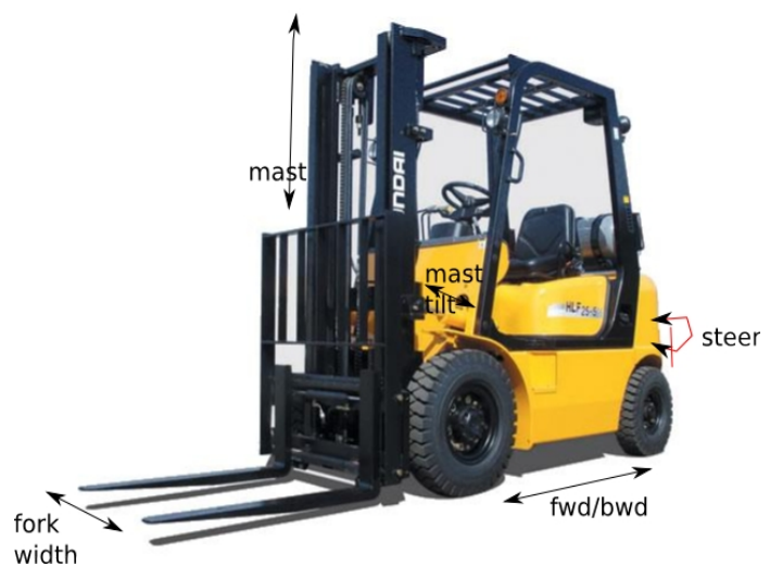
Illustration 5: Axes present in typical forklift (“Forklift,” n.d.)
