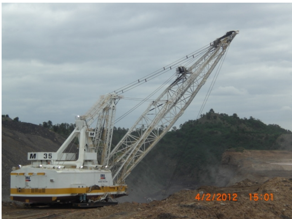
Illustration 1: A Marion 8050 Dragline in operation, conducting pre-strip of overburden. To estimate scale, note the size of the standard walkways on the side of the machine.
