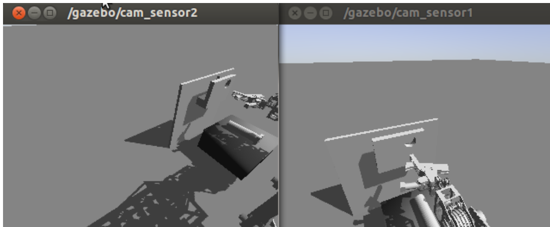
Illustration 10: Camera Configuration 2, two head cameras providing some depth perception
