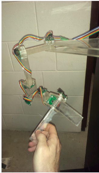
Illustration 13: Master Arm Interface showing Joints
