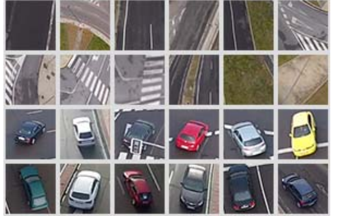
Fig. 2. A subset of the training data used for the CNN, where the dataset is divided into two classes: background (first and second rows) and target (third and fourth rows)
