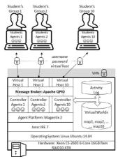
Fig. 3. Arquitecture of the virtual laboratory for distributed multiagent systems. It is supported by a Xeon server with a double security barrier. Students's groups must both connect through the University's VPN, and provide an additional username and password to connect to their own multiagent system. All multiagent systems in the server log all the transactions and have access to several virtual worlds
