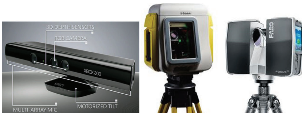
FIG. 2—Laser scanners used for the experiment. From left to right: Kinect, Trimble, and Faro.
