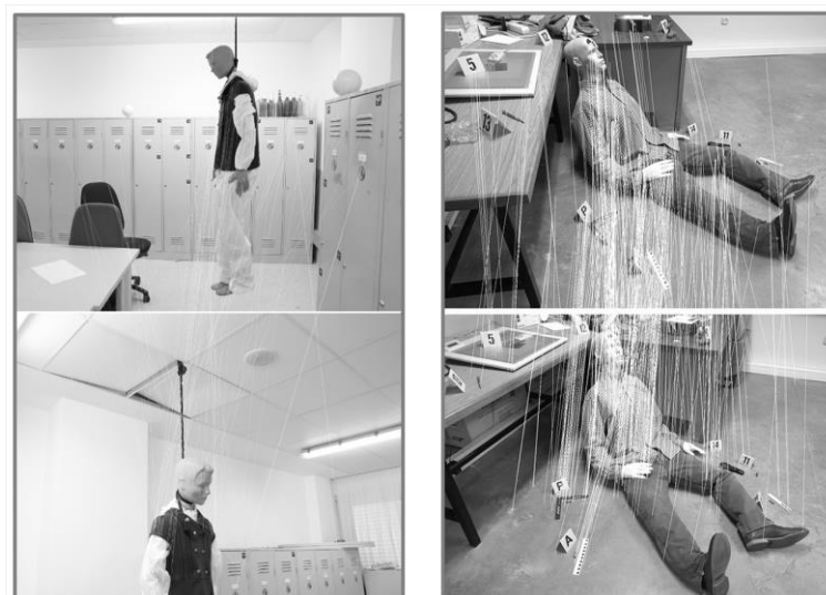
Figure 4. Matching results based on the ASIFT algorithm for a couple of images corresponding to the first crime scene, the suicide (Left) and to the second crime scene, the homicide (Right). These images show the matched points joined with a “white” line.
