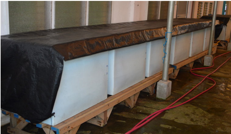
Figure 29. Double-layer black plastic is used to reduce light intensity in the rearing tanks
