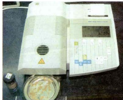
Figure 6.2 A moisture balance used to determine moisture content of feedstuffs and aquafeeds.
