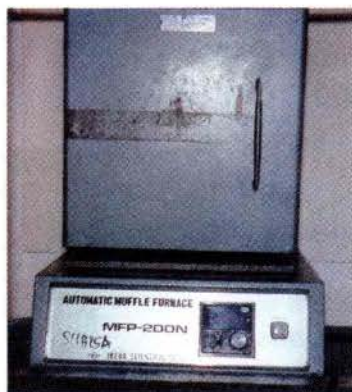
Figure 6.5 A muffle furnace used to analyze the ash content of feedstuffs and aquafeeds.
