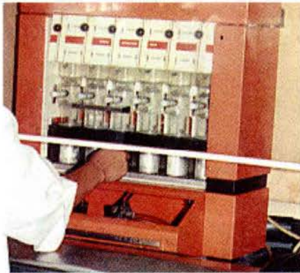
Figure 6.4 The Soxtec™ apparatus used for crude fat analysis.
