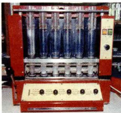
Figure 6.6 The Fibertec™ used for crude fiber determination.
