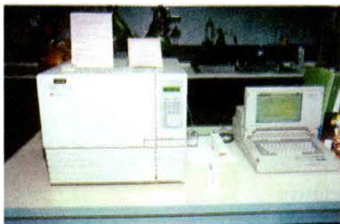
Figure 6.8 The gas chromatograph (GC), an instrument used for analysis of fatty acid composition.
