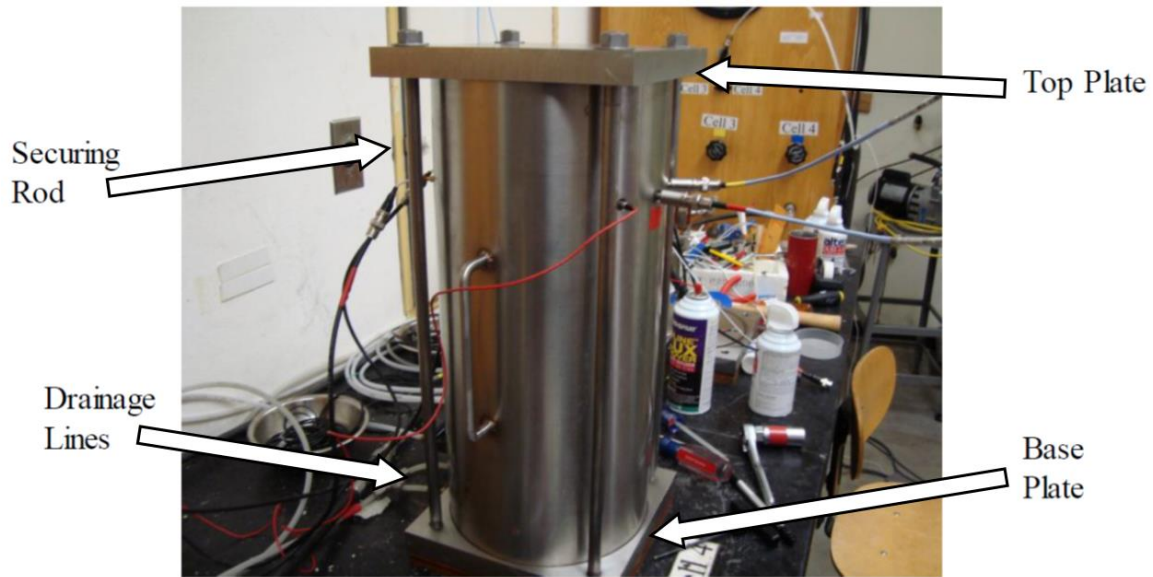
Figure 3.2 Photograph of Confining Chamber Used in RC Testing at UT (from Umberg, 2012)
