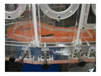
Figure 2.11: Image of Interface Slot to hold Test Articles
