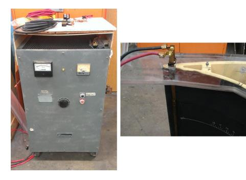
Figure 2.15: DC Power Supply (left) and Connection to Test Article B (right)
