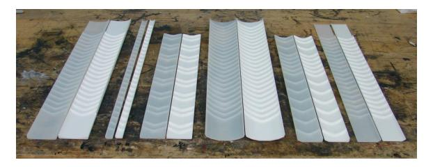
Figure 2.31: Rib Turbulators, Nylon (left) and Corian (right)
