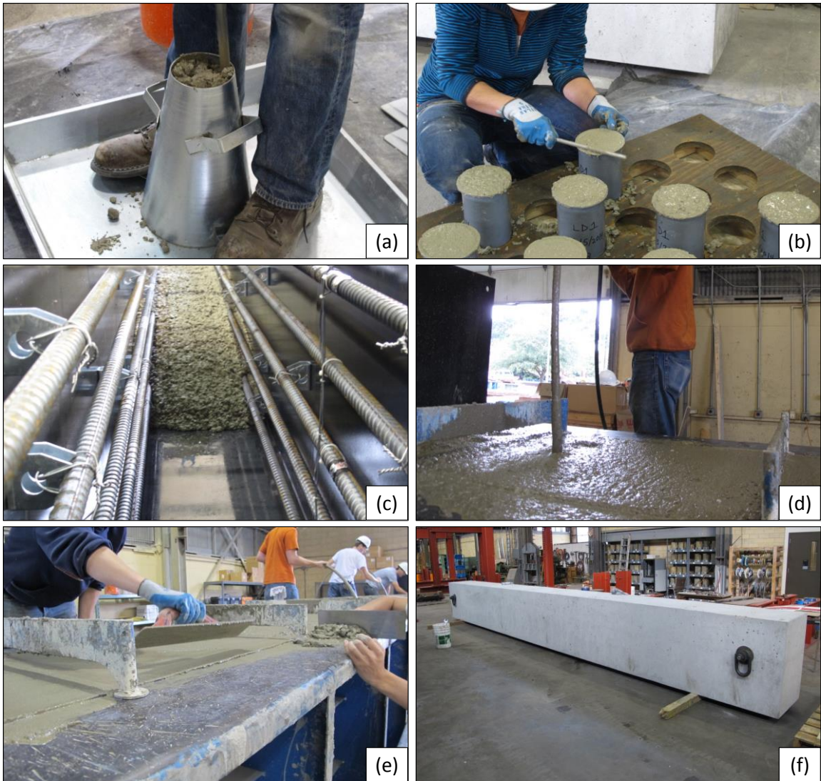
Figure B-4: Concrete Placement Showing the Following: (a) Slump Test, (b) Cylinder Finishing, (c) Main Specimen Placement, (d) Internal Vibration, (e) Finishing of Main Specimen, (f) Completed Specimen
