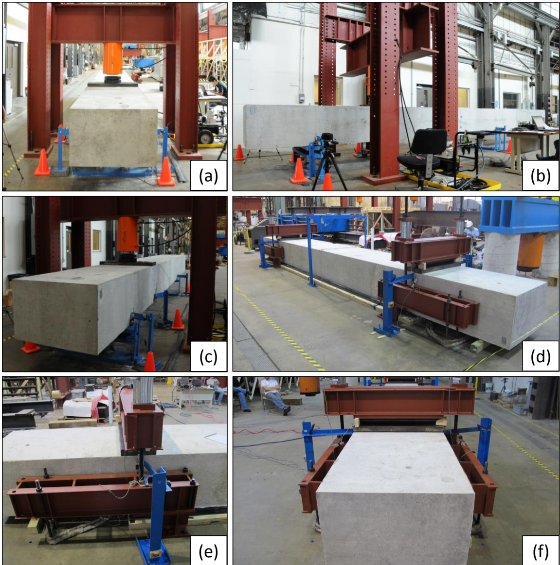
Figure B-8: Test Setup Photos Showing the Following: (a), (b), and (c) Concentrated Load Setup, (d), (e), and (f) Uniform Load Setup
