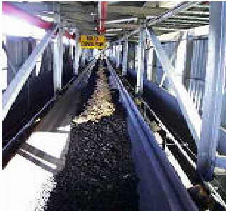
Figure 13.1 A Blended-Feed Co-Firing System
