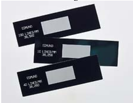
Figure A.1: Ronchi ruling from Edmond Optics ( http://www.edmundoptics.com )
