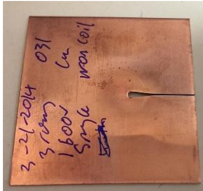
Figure 5.10. An annealed copper 110 sample where deformation at the starter notch was observed.
