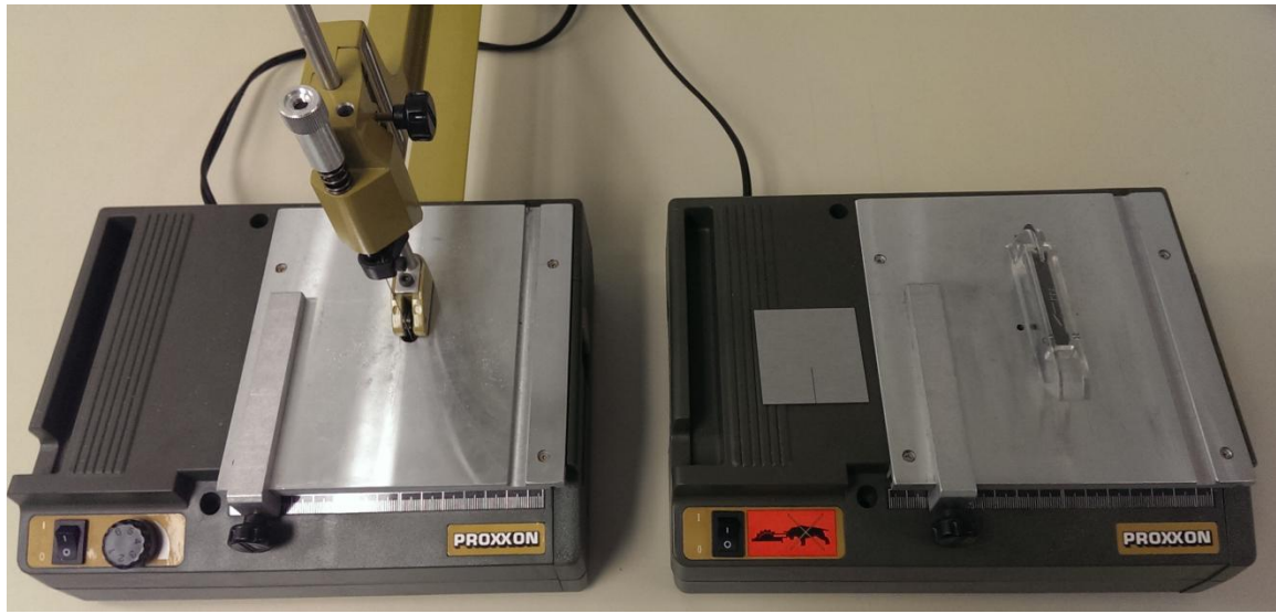
Figure 5.15 Two small saws used for model building. These saws can use blades as thin as 0.13 mm and were procured to investigate the possibility of using them to make the starter cuts. A standard size sample can be seen on the radial saw.
