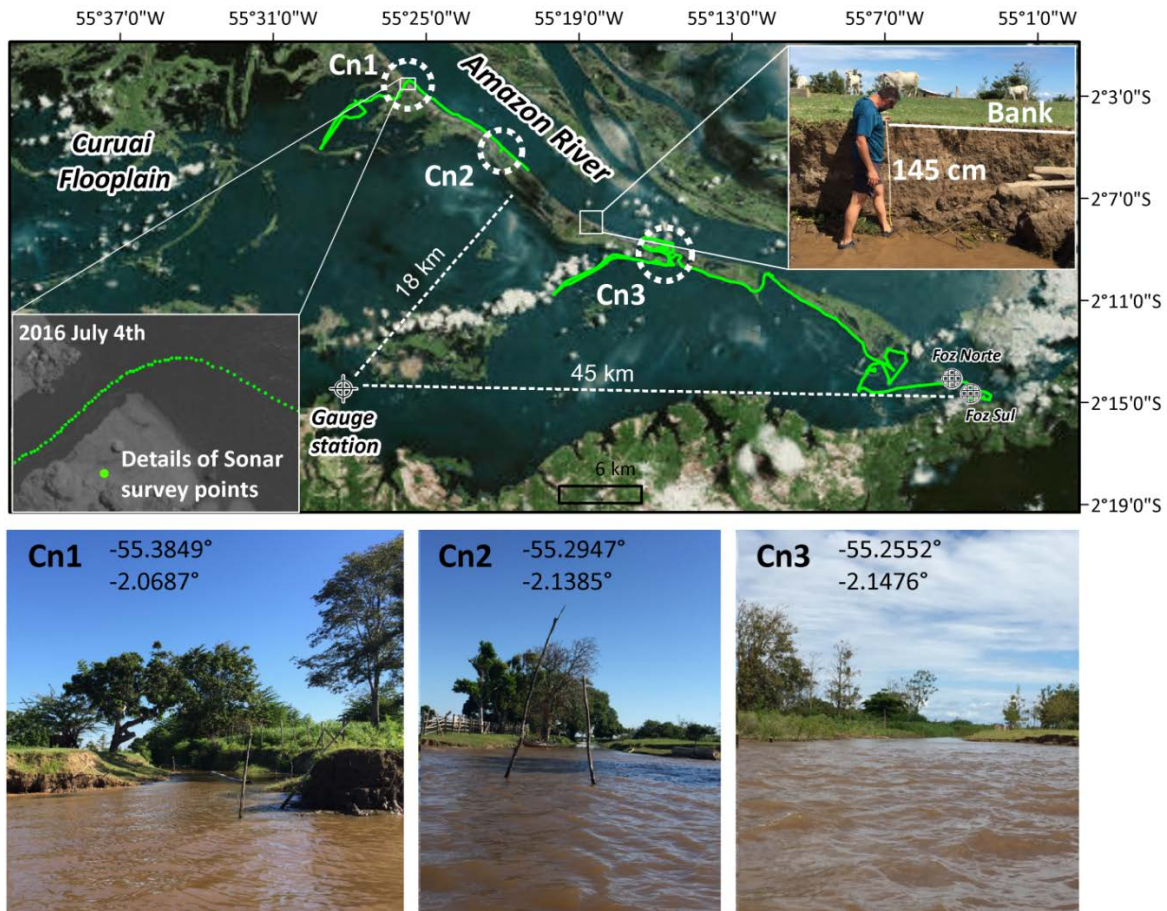
Figure 4.3. Verifying the channel-floodplain connectivity water level threshold (540 cm) at Obidos identified in Figure 4.02a. Sonar bathymetric survey routes along the Amazon River right bank on July 4 th , 2016. Three channel-floodplain hydrological connections (Cn1-3, indicated as white dashed-circles) are identified, where the pictures of their entrances from the river are also shown. Inset picture shows Maxi Bayer measuring the bank height above water level during the field work.
