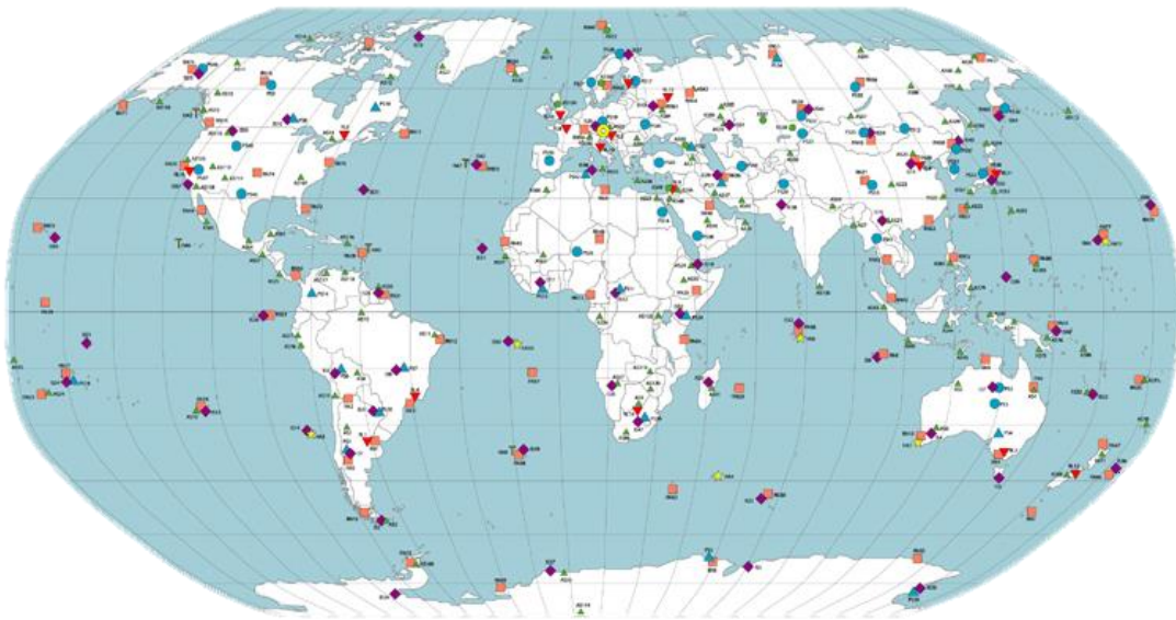
Figure 2: Locations of the IMS stations. All blue and green points are seismic stations. The shape and color identify the specific type of seismic station. The orange squares are radionuclide stations. The red triangles are radionuclide laboratories. The yellow stars and brown tees are hydroacoustic stations. The purple diamonds are infrasound stations. The yellow circle is the CTBTO International Data Centre. [1]
