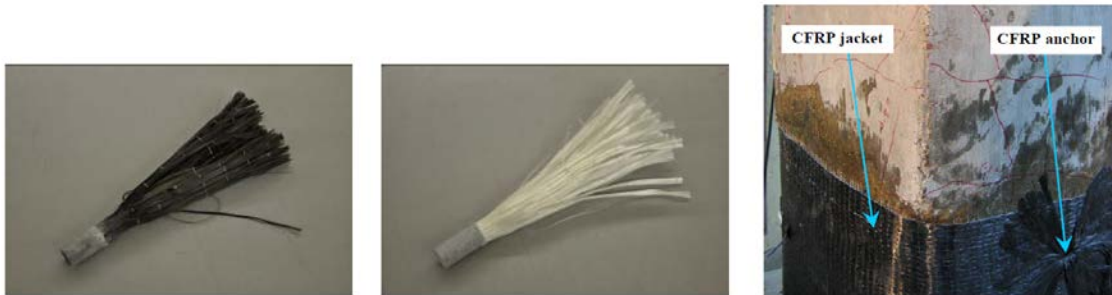
Figure 3.1: a) CFRP anchor, b) GFRP anchor, c) CFRP jackets with CFRP anchors
