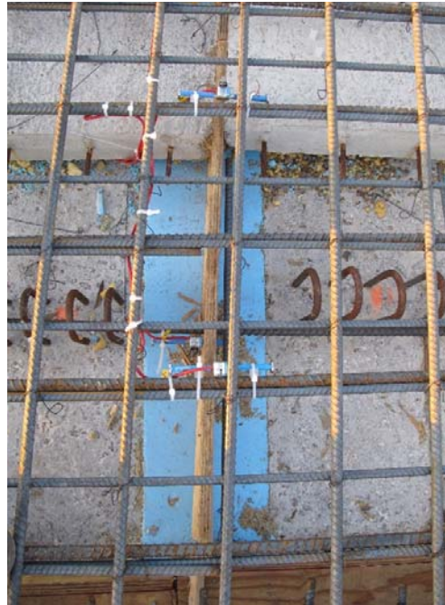
Figure 3.43: Wood Crack Former
