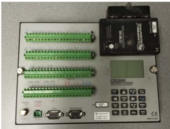
Figure 3.5: CR3000 Data Logger
