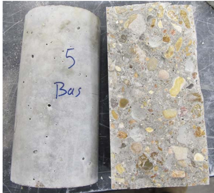
Figure 4.28: Split Cylinder Test
