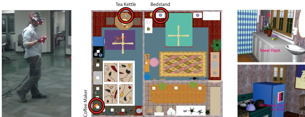
Figure 1. Subjects performed a visual search task within a virtual-reality three-room apartment. A. Subjects wore a V8 head mounted display equipped with an ASL eye tracker, while the head and hand were tracked using the PhaseSpace motion tracking system. The subject touched virtual objects in the apartment using the gloved hand when they were located. B. Overhead view of the virtual apartment showing the three rooms: bathroom, bedroom, and kitchen. The 3 objects specified for repeated search are indicated by red circles. C. Two example views, recorded while a human subject was exploring the apartment wearing the HMD. Targets were specified by words at the bottom of the screen (e.g. "Coffee Maker") and the subject had to locate and touch that object (e.g. the orange coffee maker). Gaze position, head orientation and location were recorded for later analysis.
