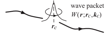
FIG. 10. The wave-packet description of a charge carrier whose center is (\mathbf{r}_c, \mathbf{q}_c) . A wave packet generally possesses two kinds of motion: the center-of-mass motion and the self-rotation around its center. From Xiao, Yao, et al. , 2006.
