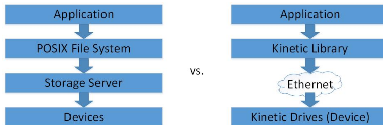
Figure 4.1: Software stack of server with traditional drives vs. Kinetic drives.
