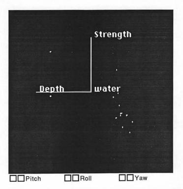
These data concern samples of thawed permafrost soil. strength is the shear strength, and water is the percentage water content. depth is the depth at which the sample was taken. The plot shows that a linear model will not fit well. Devore and Peck (1986) suggest fitting a model with quadratic terms to this data.
