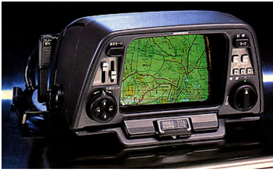
Figure 8. Honda Electro Gyrocoator. Reprinted from Hand-Cranked Maps to the Cloud: Charting the History of In-Car Navigation , by Newcomb, D., 2010. Retrieved from https://www.wired.com/2013/04/history-in-car-navigation/
