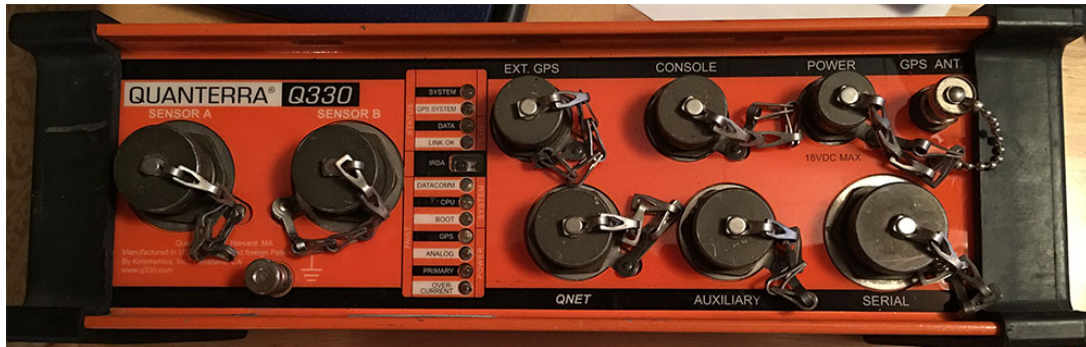
Figure 6.4: Quanterra Q330 Digitizer. The seismometer is connected through one of the SENSOR ports on the left. A GPS antenna may be connected to the GPS ANT port. The Quanterra B14 Packet Balers were connected through the SERIAL port. The Q330 is powered either by the POWER port or the QNET port. The Q330 can be connected to a local network, or a local radio antenna, via the QNET port.
