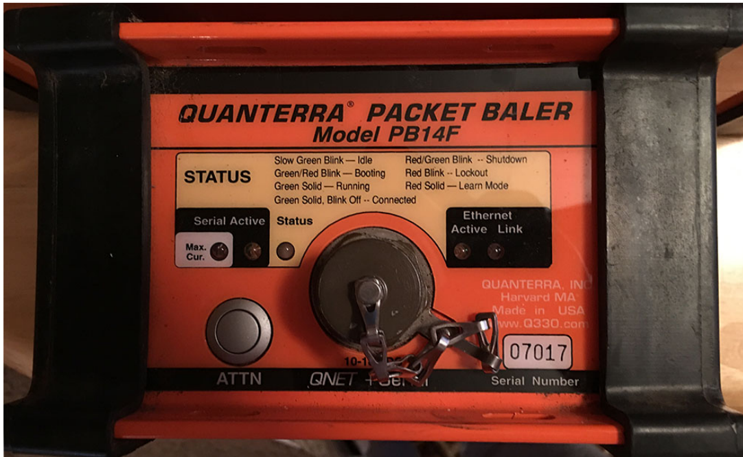
Figure 6.5: Quanterra P14 Packet Baler. The QNET serial port is used to connect to the Q330. The ATTN button will turn on the baler and request that Q330 buffer dump its data to the baler.
