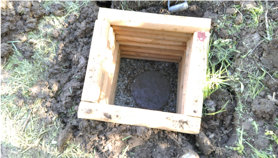
Figure 6.6: An example of a the small enclosure that housed the surface station seismometers.
