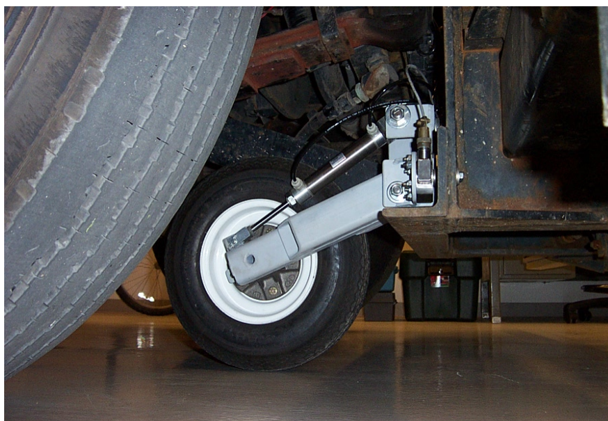
Figure 1: Friction measurement wheel installed on a snowplow.
