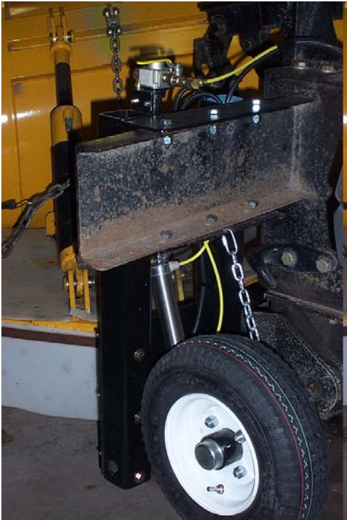
Figure 12: Friction wheel installed on the second Polk County snowplow.
