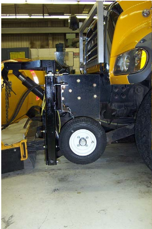
Figure 10: Side view of friction wheel installation on the first truck with the wheel in the raised position.
