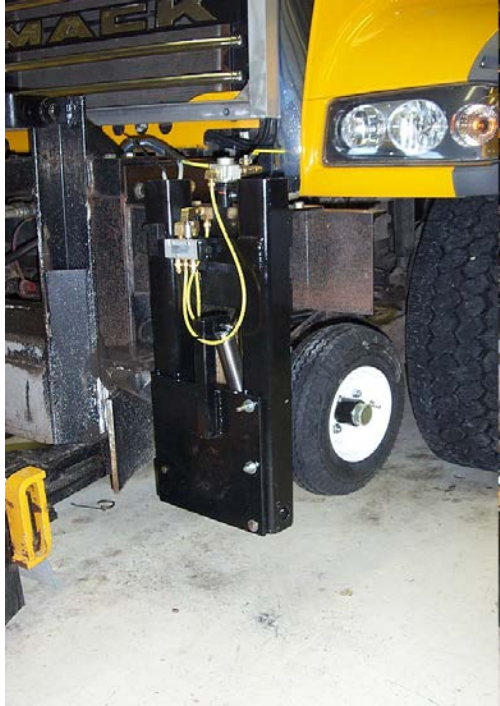
Figure 9: Complete road friction sensing system installed on the first of two Polk County snowplows.
