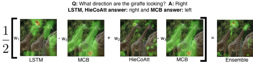
Figure 6.3: The Penalized Weighted Average (PWA) ensemble explanation approach on an instance of the VQA data. In this case, the LSTM and HieCoAtt systems agree with the ensemble’s answer (i.e., “right”) while the MCB disagrees.
