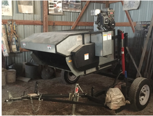
Figure 4. Mechanical seed stripper for harvesting prairie seed.
