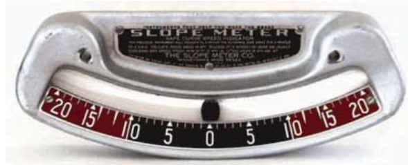
Figure 2.2 Conventional ball bank indicator (Cornell University, 2014).
