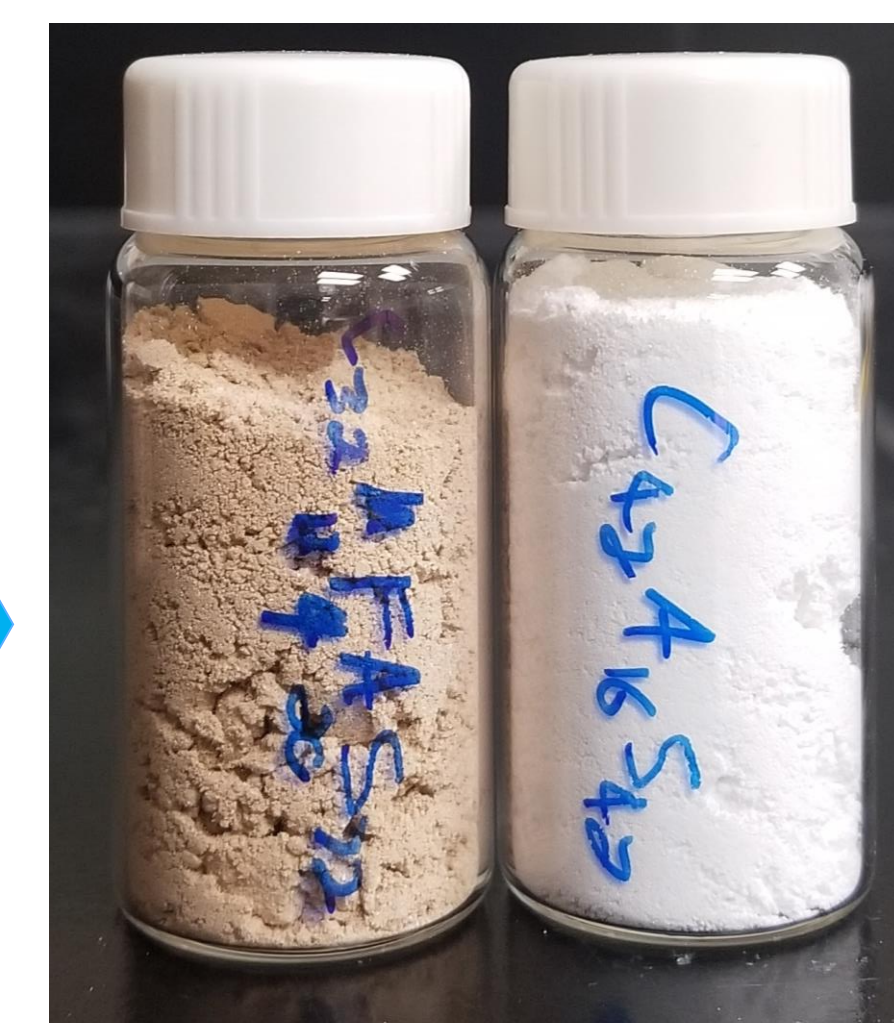
Fig 4: Calcined powder mixture to homogenous pre-reacted silicate (left). Effects of incipient melting during pre-reaction (right).
