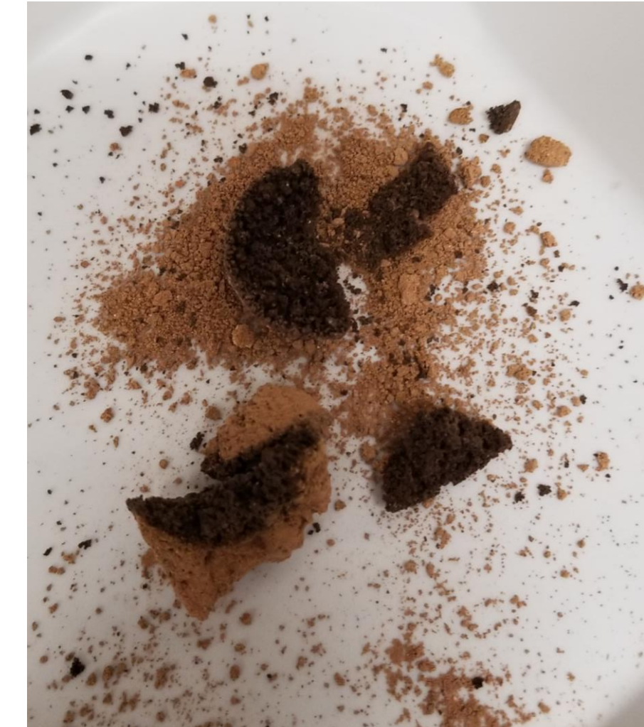
Fig 4: Calcined powder mixture to homogenous pre-reacted silicate (left). Effects of incipient melting during pre-reaction (right).
