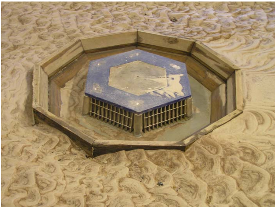
Figure 4.14. Bed topography around the original geometry looking from the Virginia shoreline (same angle as in Figure 4.13).
