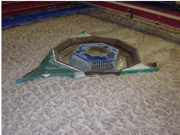
Figure 1.2. Sixth geometry: A long nose wall, with wingwalls, and a crown around the nose wall, the sand barrier and the wingwalls. In this figure, the crown was removed to scan the bed forms around the structure.
