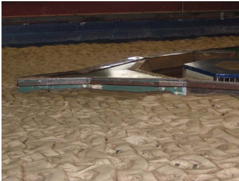
Figure 4.18. The screen installed at the mid height of the wall around the structure.
