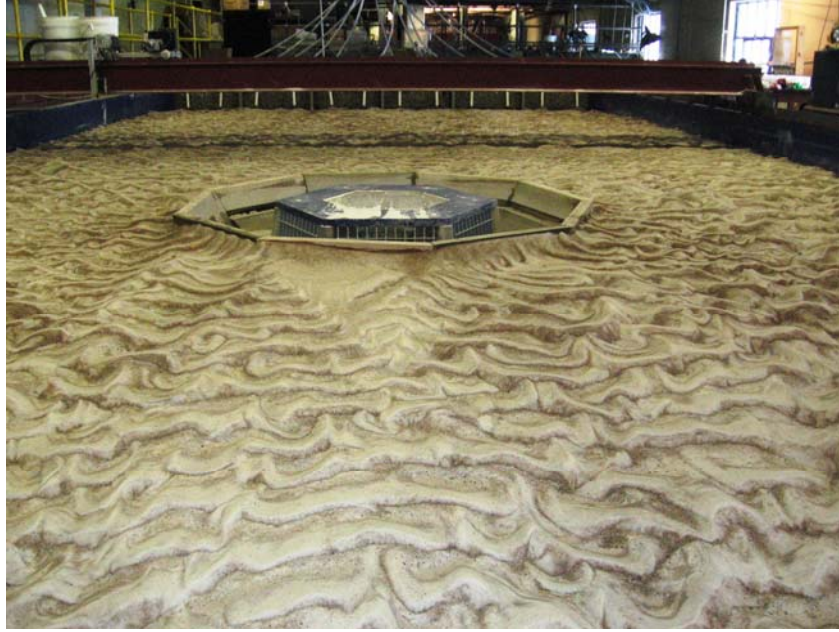
Figure 2.1. The original geometry and the bed forms created at the model scale.
