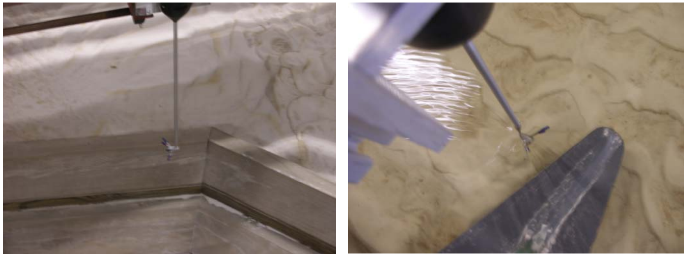
Figure 2.2. The Nortek Vectrino+ ADV used for velocity measurement.
