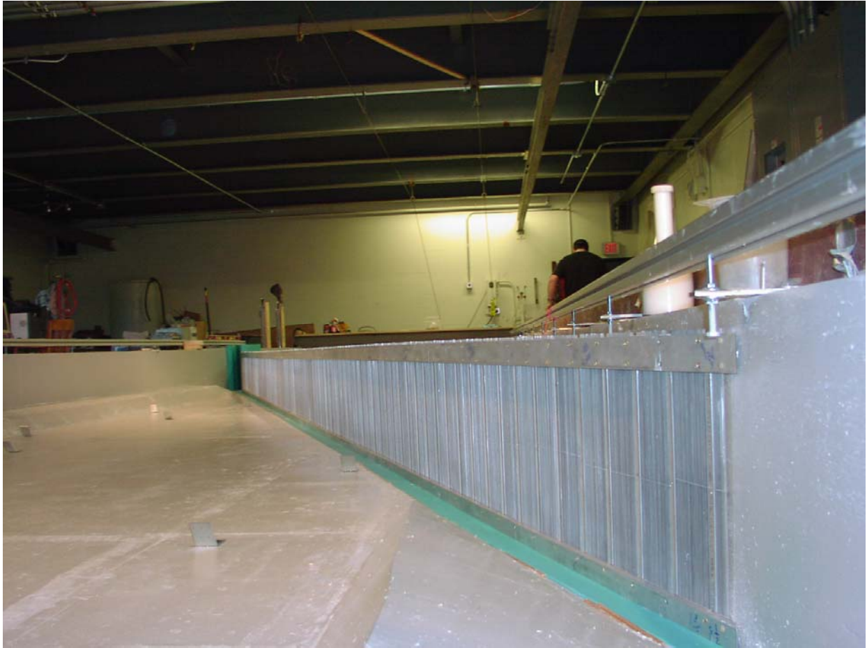
Figure 7. View of the model louver structure from upstream. The sloped board at the bottom is the eel passage.
