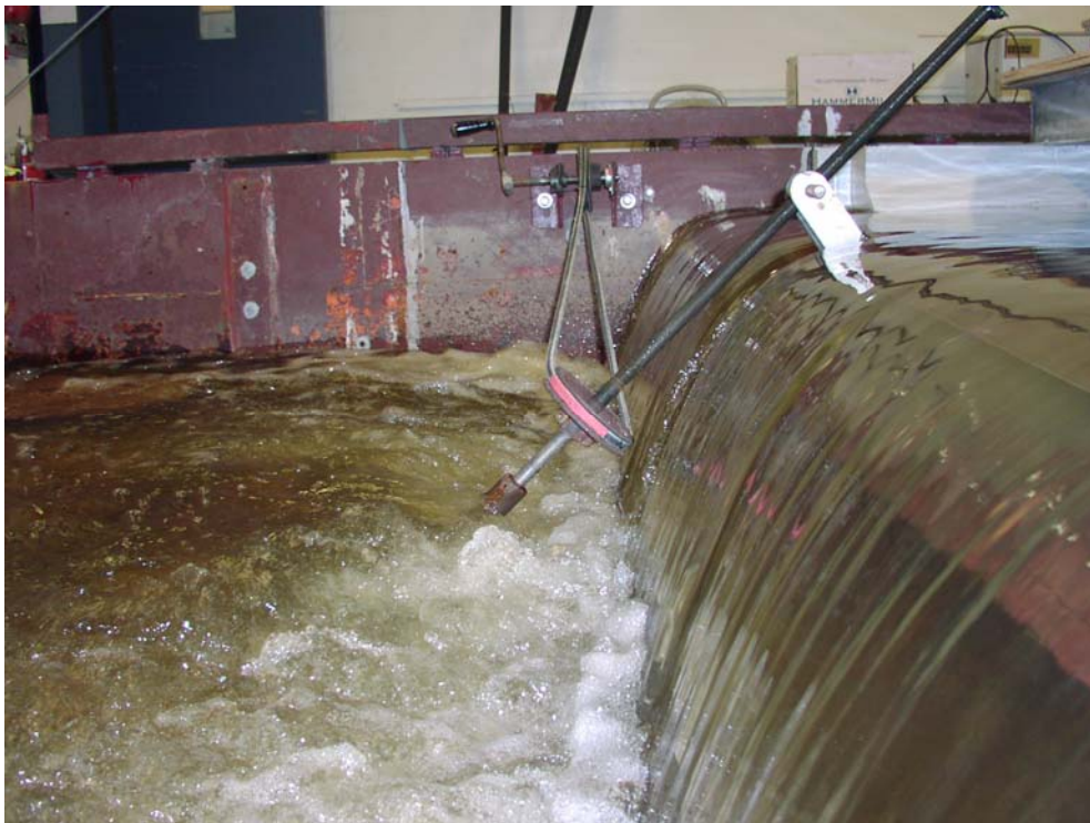
Figure 5. The tilting gate at the end of the model to control the downstream water level boundary conditions.
