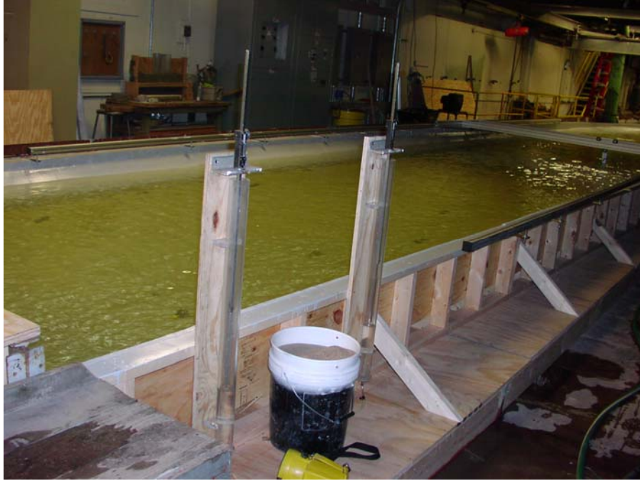
Figure 9. The wet wells for reading water surface elevations at cross-sections 14 and 13.88.
