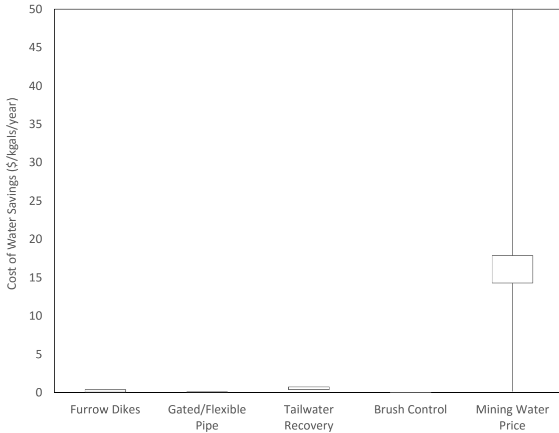
Figure 4.6: The price of water varies per BMP, but all water conservation measures cost less than the wholesale price of water for hydraulic fracturing in Texas. The box plot of water price shows the 1st and 3rd quartiles within the boxes. The lines extending beyond the box, or whiskers, show the data outside of those quartiles. The price paid for mining water does not include transaction costs which vary regionally. (Figure created by the authors based on analysis and data from private operators and [1–20, 23]).
