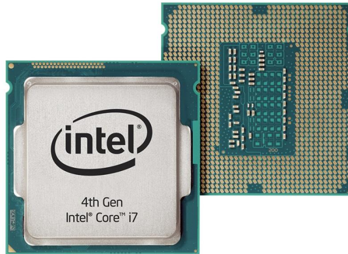
Figure 4.4: The Intel Core i7-4770K, a modern microprocessor housed in a flip-chip LGA package. The die is concealed by the large metal heat spreader. 175
