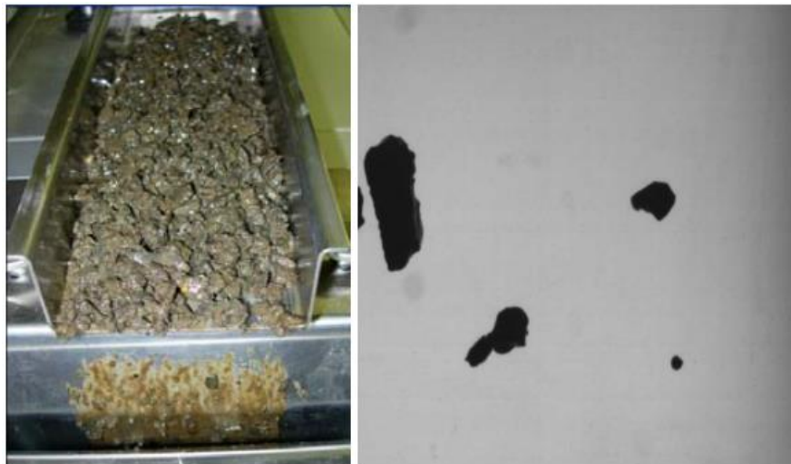
Figure 2-5: Analysis of cuttings morphology. A trail of cuttings sample (left) and cuttings under 2D camera (right)(Omland, et al. 2007).
