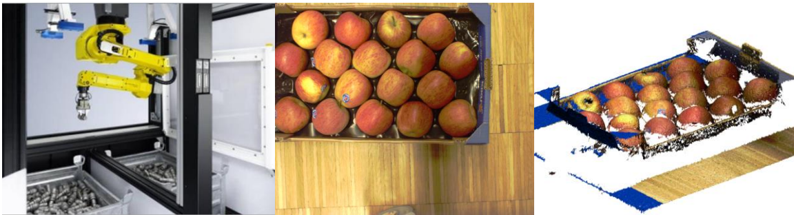
Figure 5-5: (Left to right) a) Sensor mounted on a moving robotic arm b) RGB image c) 3D point cloud profile of objects (IDS, Obtaining Depth Information from Stereo Images - Whitepaper 2012)
