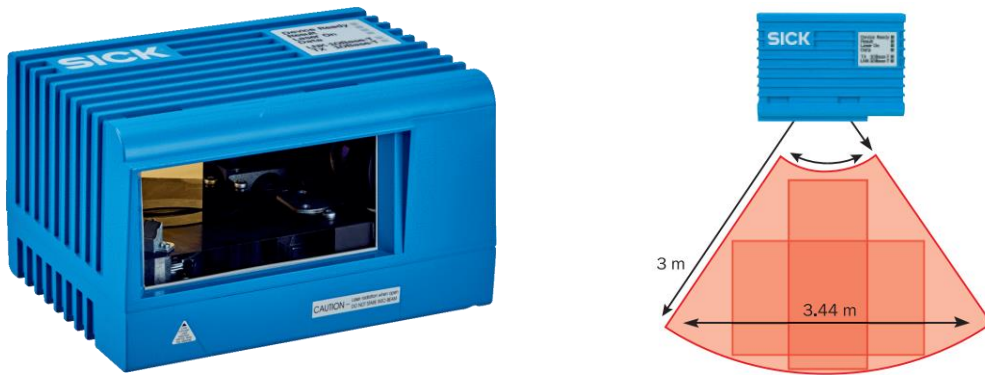
Figure 5-6: SICK LMS400-2000 laser scanner (left) and field of view (right) (SICK, LMS400-2000 Data Sheet 2012)
