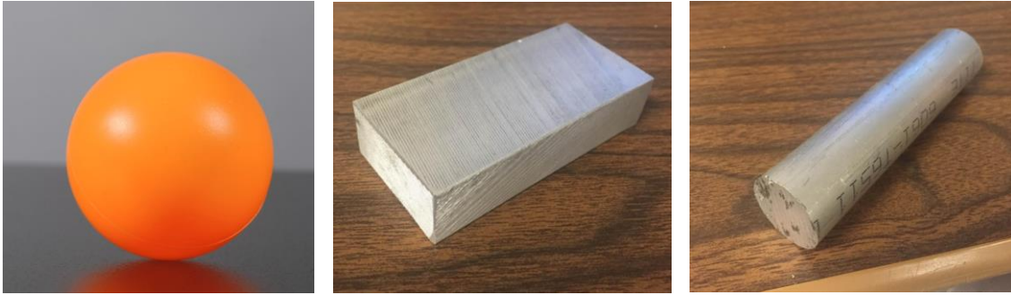
Figure 5-29 a) Ping-pong ball (Sellercube 2016) radius = 40mm b) Aluminum bar (15mm x 30 mm x 70mm) c) Aluminum rod (OD= 25 mm, length = 100 mm)
