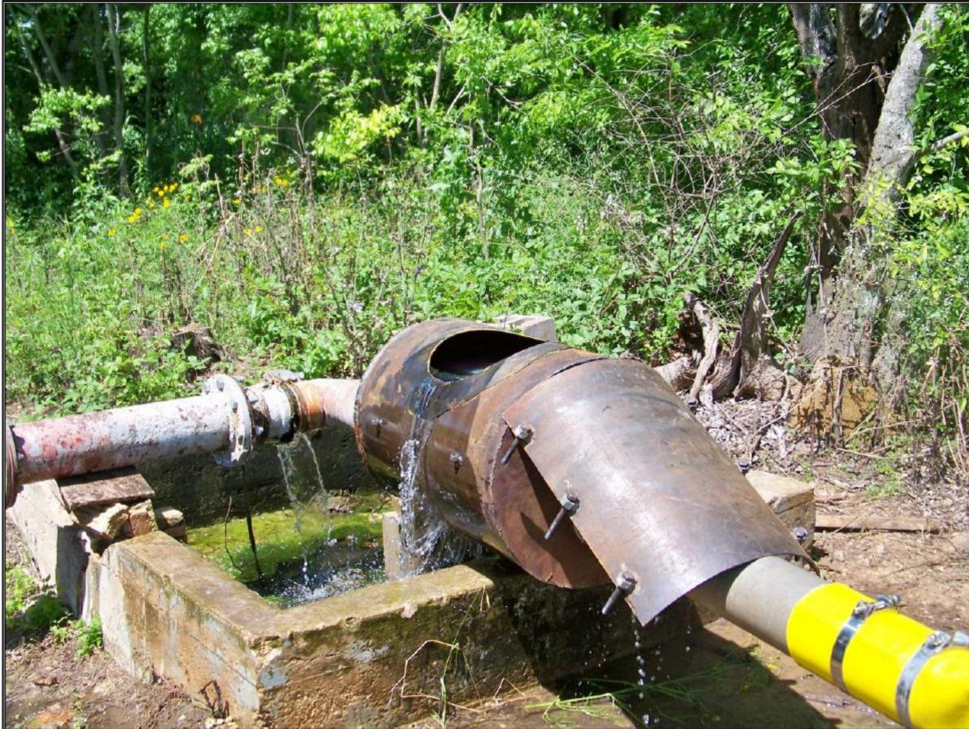
In line barrel sampler on an irrigation well in Bexar County, Texas.
