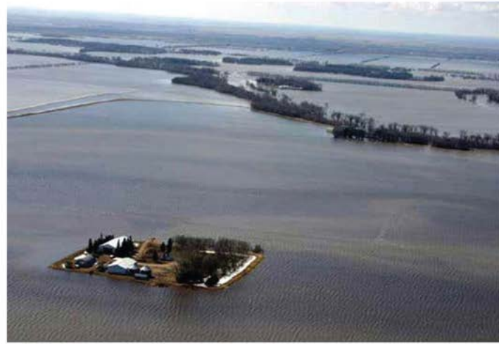
Flooding of farmland. The farmstead is protected by a ring dike. © MSTRWD.
