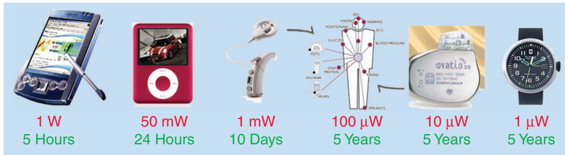
Figure 1.1: Typical power and lifetime requirements of small electronic products incorporating wireless sensor networks [3]
