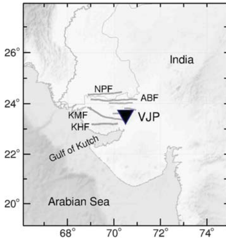
Figure 9. A plot showing one three-component broadband seismograph station. Stations (black solid triangles): VJP, Vajepar. Major faults (lines): ABF, Allah Bund fault; KMF, Kachchh mainland fault; KHF, Katrol Hill fault; NPF, Nagar Parkar fault.
