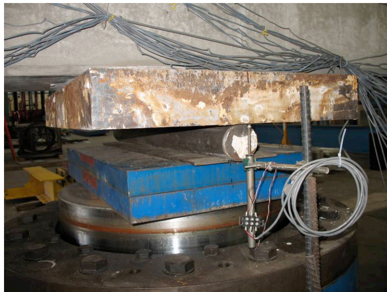
Figure 3-27. Linear potentiometer used to measure the displacement at the load point.
