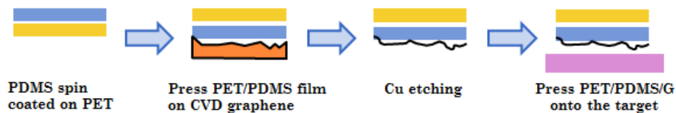
Figure 3.4 Schematic illustration of graphene transfer with cured PDMS on PET
