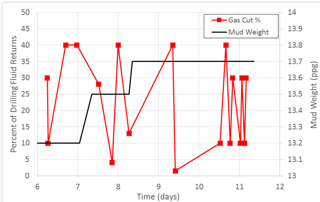
Figure 3.7: Mud weight and gas cuts after kick at 15,834 ft. (Data from Lage et al., 2002)
