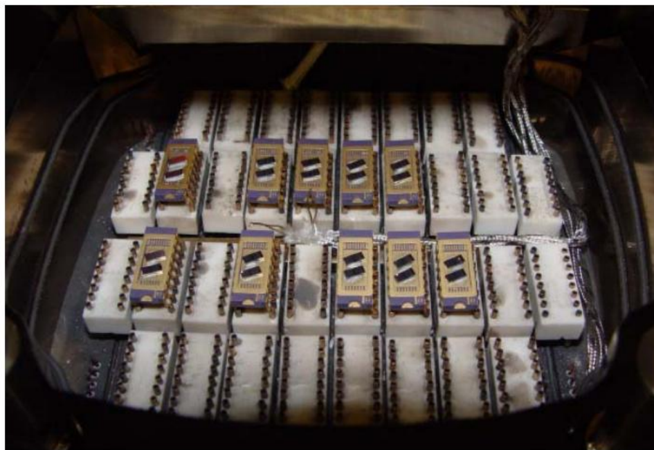
Figure 2.3 In-house package-level EM testing system with a close-up of the interior of the chamber.
