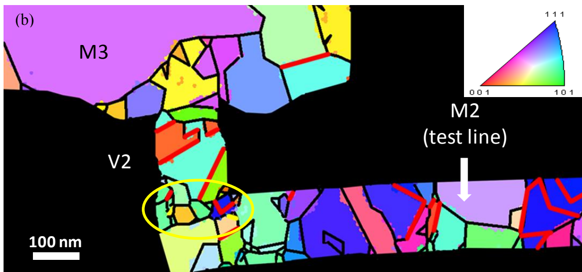
Figure 4.9 (a) BF TEM image of Cu trench (M2) and via (V2) for the 45 nm node SG structure. (b) The color coded IPF orientation map for the same via/line region.
